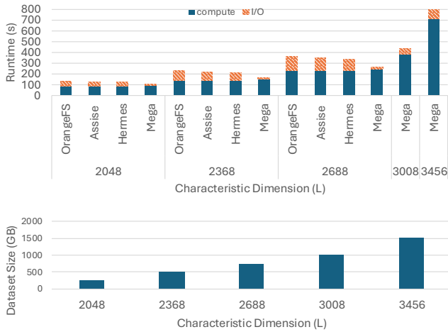
Fig. 6: Increasing the resolution of Gray-Scott through tiering. After L=2688 , MPI-based Gray-Scott crashes due to memory overutilization. MegaMmap is unbounded, and can run simulations as large as L=3456 , producing 2x the simulation data of L=2688 . It’s also at least 20% faster than other tiered I/O systems due to effective asynchronous data movement.
